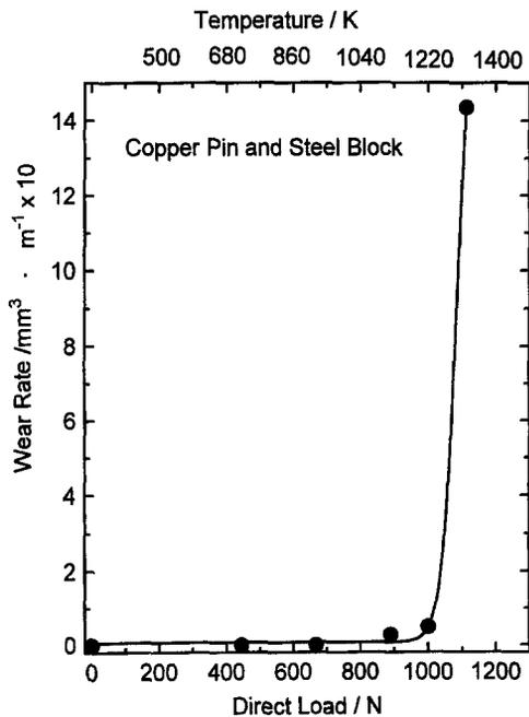
Fig. 1. Plot of removal rate (amount of material removed in 600 s) versus applied load when using a copper pin immersed in poly  $\alpha$ -olefin.
