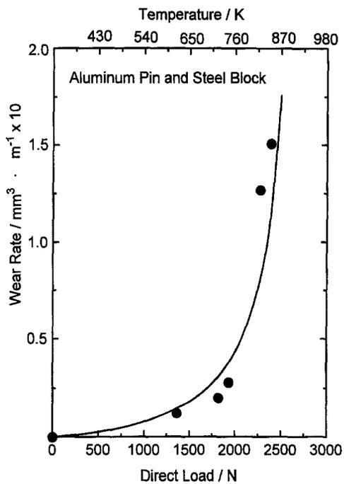
Fig. 3. Plot of removal rate (amount of material removed in 600 s) versus applied load when using an aluminum pin immersed in poly  $\alpha$ -olefin.
