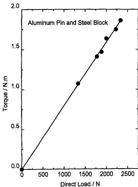
Fig. 4. Plot of torque versus load when using an aluminum pin immersed in poly  $\alpha$ -olefin.
