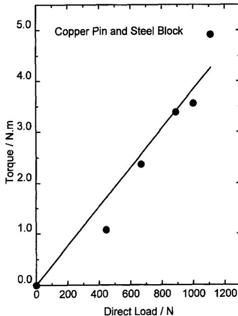
Fig. 2. Plot of torque versus load when using a copper pin immersed in poly  $\alpha$ -olefin.
